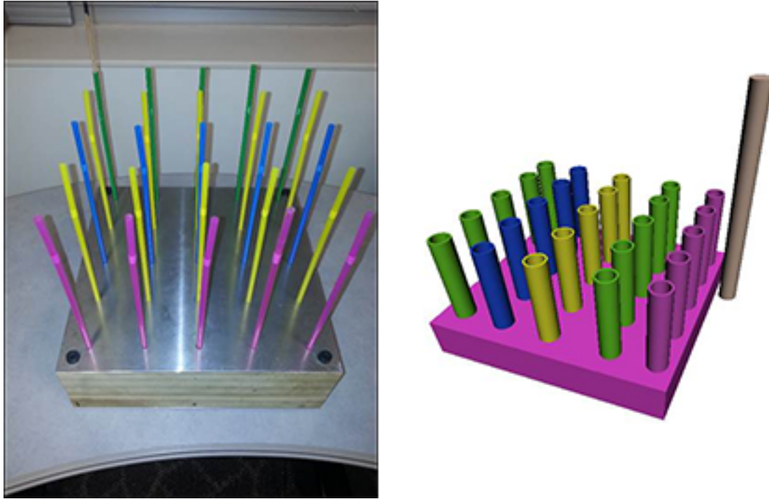
Figure 3.8 On left, the physical peg-in-hole board and on right, the virtual peg-in-hole board into which participants sequentially placed narrow dowels.
